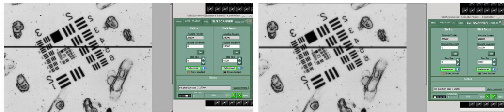
Figure 7: Left: in focus. Right: slightly out of focus (note the blurrier slit). In this case the focus test was done by moving the lens with its motor, to make sure that 24000 corresponds to the optimum focus position. This test is good once the ideal lens position is found. One can try setting the focus to 20000 and to 28000, which should lead to an equal defocus compared to 24000.
