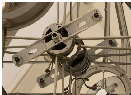
Figure 16: Two lasers for alignment mounted at the F2 flange
